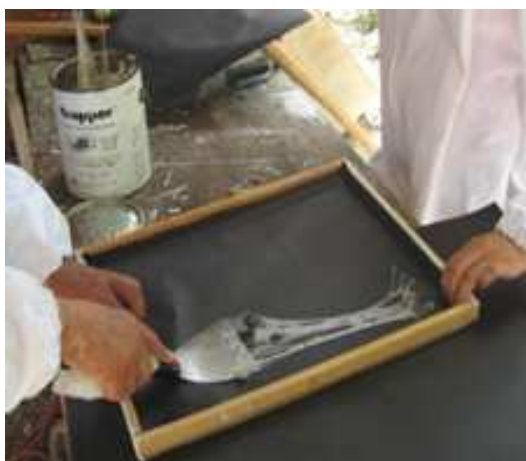
Figure 2 D. Placement of adhesive SEHU-TAK
