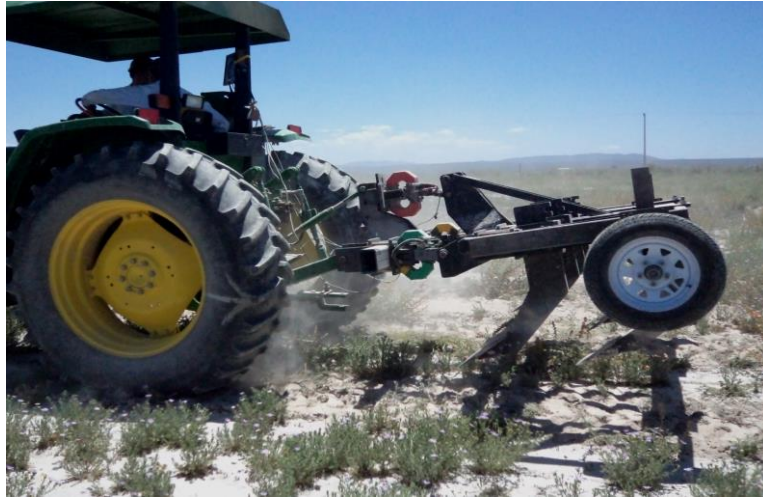
Figure 2 Apparatus set for field evaluation, showing the integral force transducer.
