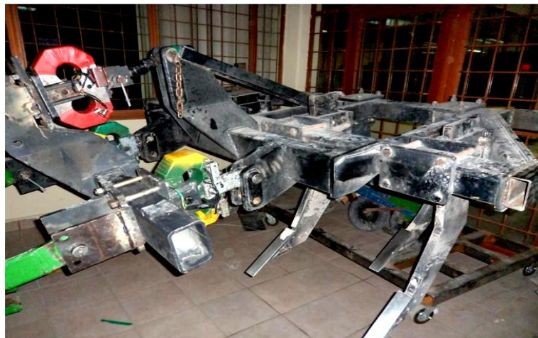
Figure 1. Integral force transducer employed during field evaluation of a prototype for vertical tillage.
